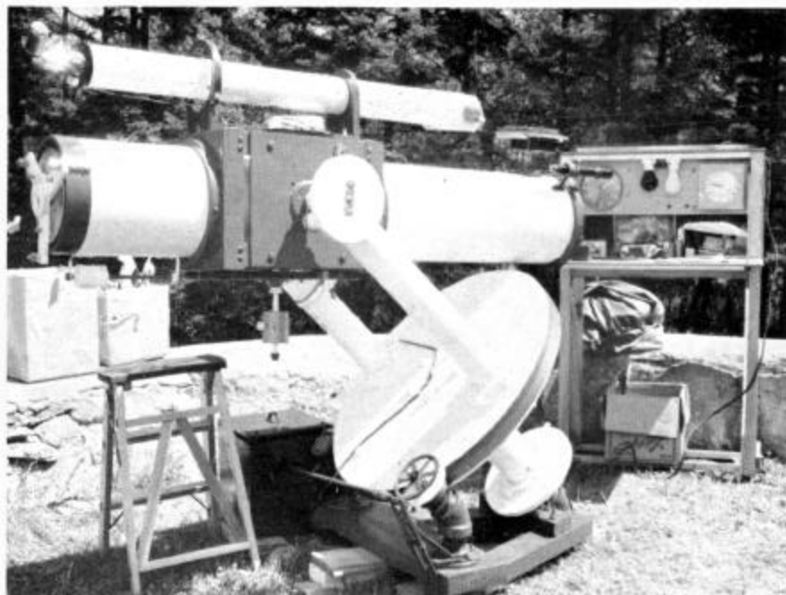
Berton C. Willard's 8-inch reflector won first prize. A counterweight beneath the main tube balances the long guiding telescope mounted on top. In the right background is the well-equipped control console. Stellafane photographs by Robert E. Cox.
