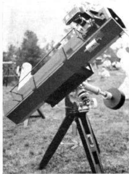
Notable among the Stellafane exhibits was this reflector, with a hexagonal wooden tube, an alarm-clock drive, and adapters for photography. It was made by Albert Nagler, New York City.
