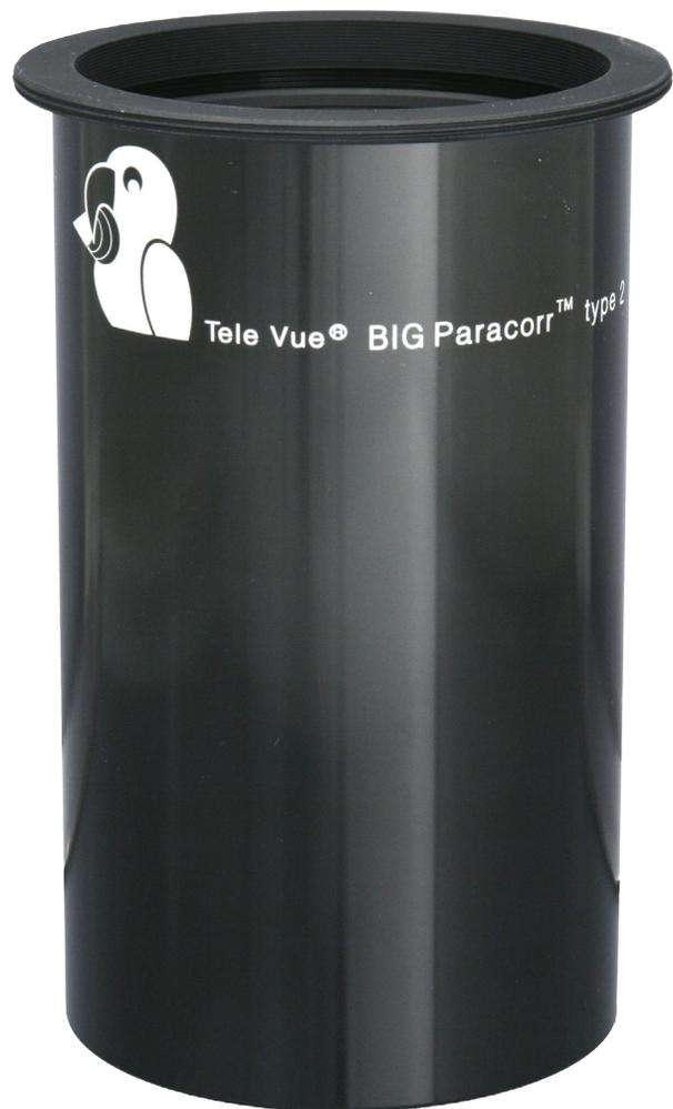
**Big Paracorr type 2** Newtonian coma corrector • 3" O.D. • 15% magnification factor • removeable top flange 3.40"-24 threads • 80mm Back Focus • Prime Focus moves 72.3mm out from native focus position • Weight: 24 oz. • Length to base of flange: 5.1"
